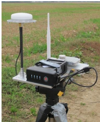
RTK GNSS Base station
